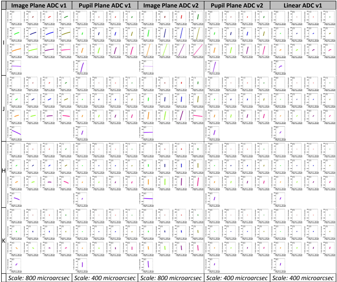
Figure 50. The layout of the 20 plots above is similar as in Figure 49: From top to bottom the different bands are shown: I, J, H and K-band. The plots, from left to right are for the first ADC study counter-rotating image plane ADC, the first ADC study counter-rotating pupil plane ADC, the current counter-rotating image plane ADC, the current counter rotating pupil plane ADC and an image plane Linear ADC. Notice the difference in scale between the various plots, as indicated by the full size of the plotted box on the bottom row of the table. In the above 8 plots the residual chromatic error is shown for one of the points at the edge of the MICADO field. The residual chromatic error is the wavelength dependent distance between center and corner point. What is shown in the 13 sub-plots is the difference between the effect a zenith distance of 0 and given zenith distance from 0 up to 60 degrees at 5 degree interval. Each point indicates the position of a different wavelength within the band, creating a line or curve.
